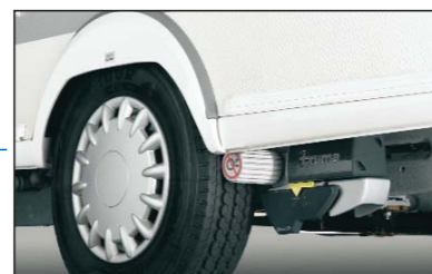
Mover SE and TE engages and disengages electronically at the touch of a button
